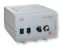
The F.O. Projector HK 7000 incorporates a special long-life halogen bulb rated at 150 Watts. If more light is needed for a particular examination, a boost switch can be operated, giving up to 40% more light. Suitable for all HEINE Systems with fiber optic illumination. Dimensions: Width 177 mm, Height 125 mm, Depth 217 mm. Weight 3,690 g.
